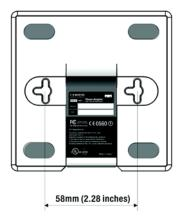
Figure 3-7: Measurement between Wall-Mount Slots
