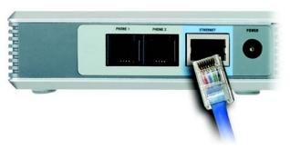
Figure 3-3: Connect the Ethernet Network Cable
