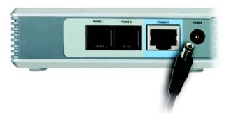
Figure 3-4: Connect the Power
