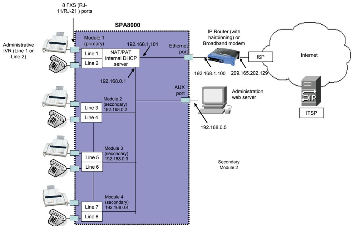
The four modules are interconnected through an internal IP network, configured automatically as a single subnet, which by default is assigned the network address 192.168.0.0 with a subnet mask of 255.255.255.0. If a network conflict is detected from the device connected on the AUX port, the internal network is automatically changed to 192.168.1.0.
