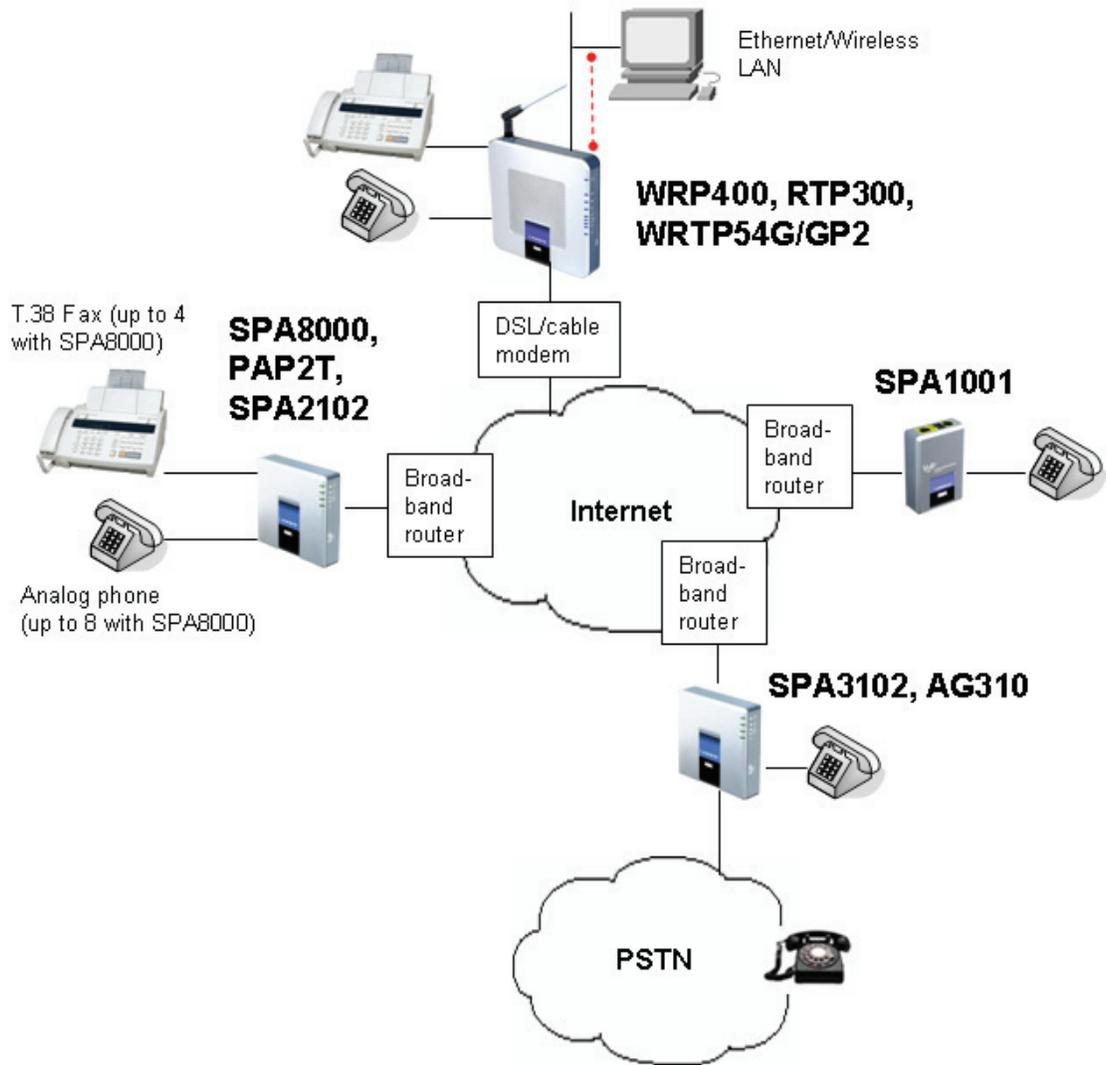
The AG310 and SPA3102 provide full PSTN connectivity in addition to a single FXS port. In addition, the AG310 provides an ADSL2+ gateway.
